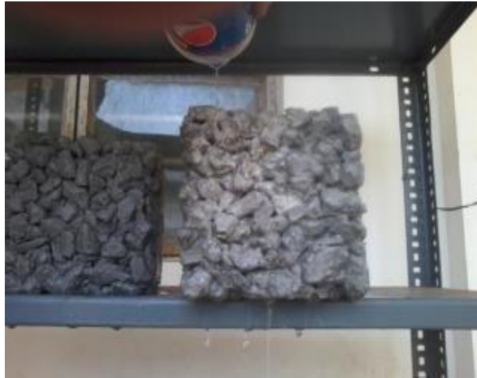
Figur1.2: Water flowing through pervious concrete cube.
