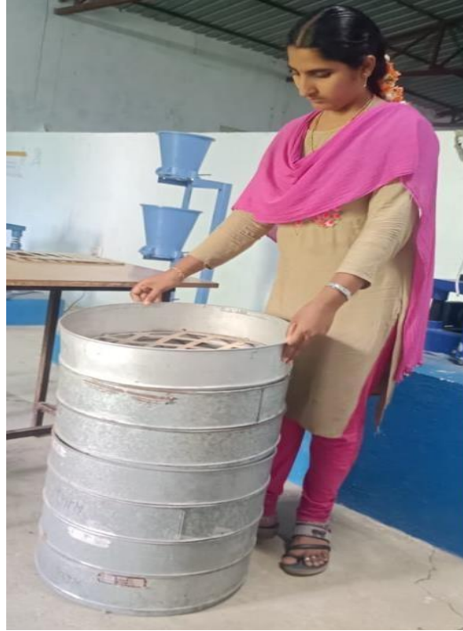
Fig 3.2.1 grading of coarse aggregates
