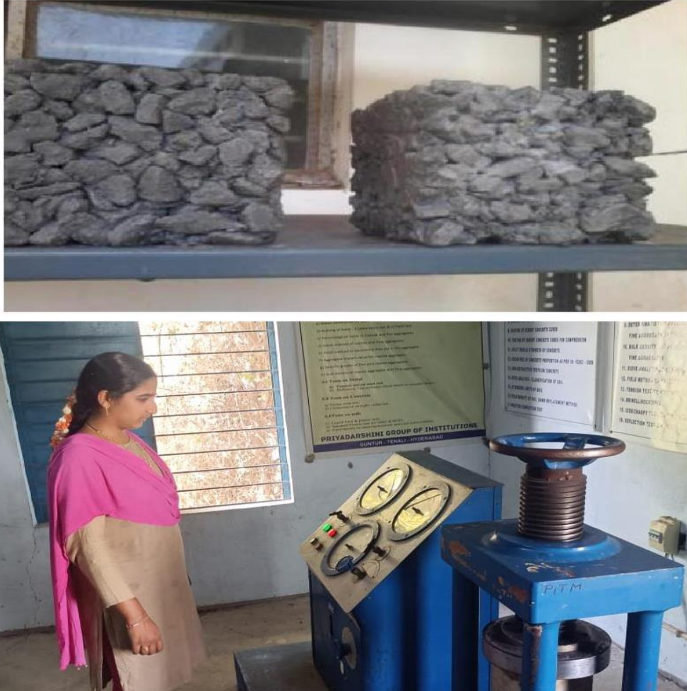
Figure3.14: Cubes tested for compressive strength.
