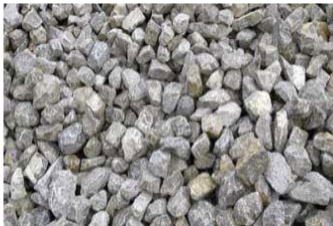
Figure 3.2 20mm coarse aggregates.
