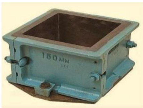
Figure3.11: Standard compressive strength cube mould.
