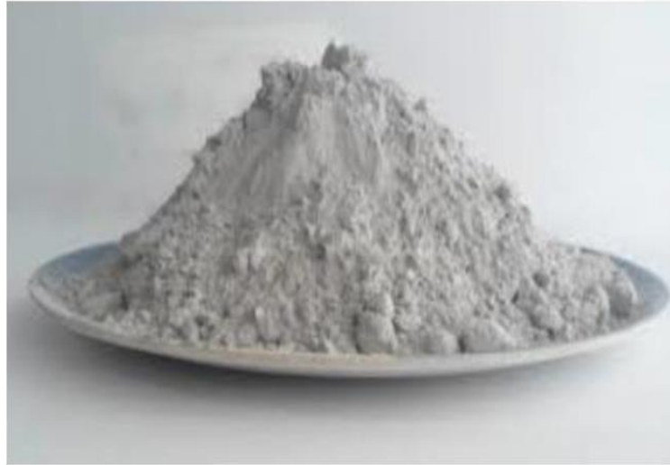
Figure3.7: Fly ash used as cement replacement.
